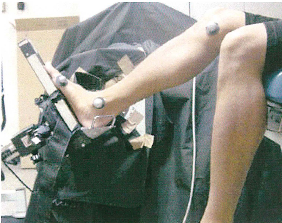
Figure 2. Reflective markers representing ankle joint center in the sagittal plane
