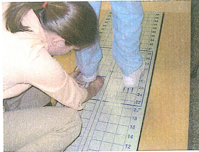
Figure 3. The subject's feet are being centered on the Balance Master®.
