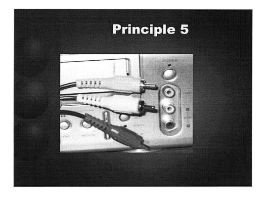
Cables which are color coded to match their connections provide a fail safe way for individuals to operate the product by eliminating complexity.
