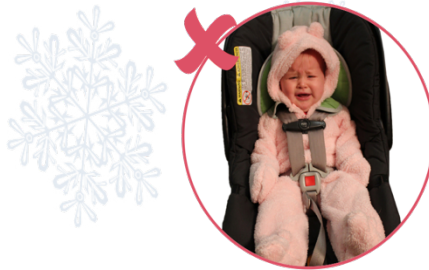
The fluff of a bulky winter coat or snow suit can compress in a car crash making harness straps loose, which can cause injury or ejection.
