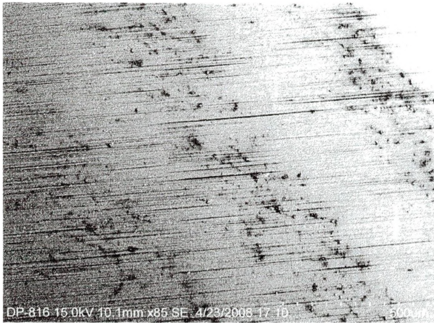
Figure 54 Specimen Testing Surface (Untested)
