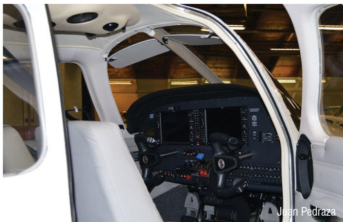
UND's latest fleet addition: one of three Piper Seminoles equipped with Garmin 1000 all-glass cockpits and the Appareo Systems flight data recorder.
