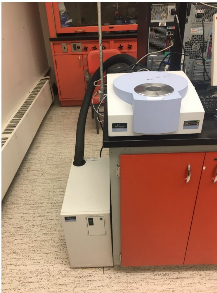
Figure 9. Photograph of the PerkinElmer® Jade DSC
