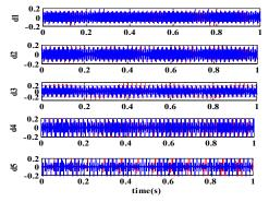
Fig.7. First test of experimental stator current details from the lifting method in healthy and faulty machine at no load with outer raceway defect (s=0).
