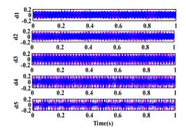
Fig.8. Second test of experimental stator current details of the lifting method in healthy and faulty machine at no load with outer raceway defect (s=0).
