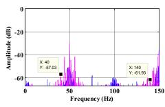
**Fig.10**. Second test of d2 of stator current spectrum of healthy and faulty motor at no load by the lifting with outer raceway defect (s=0).
