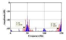
**Fig.9**. First test of d2 of stator current spectrum of healthy and faulty motor at no load by the lifting method with outer raceway defect (s=0).
