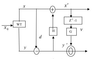
Fig. 4. Three-stage lifting scheme
