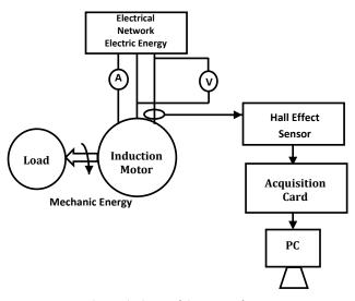
Fig.6. Electrical scheme of the circuit of experiment.
