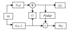
Fig. 3. principle of lifting scheme, with update step first, then with a nonlinear prediction step.
