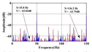
Fig.13. First test of d2 of stator current spectrum of healthy and faulty motor at full load by the lifting method with outer raceway defect (s=0.044).
