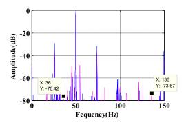
Fig.16. Second test of stator current spectrum of healthy (blue) and faulty (purple) motor at full load by FFT technique with outer raceway defect (s=0.044).
