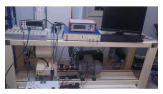
Fig.5. Experimental setup for outer race defect
