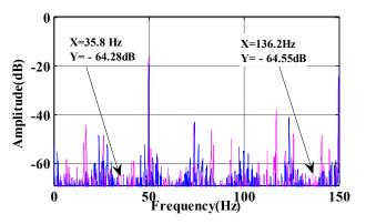
Fig.14. Second test of d2 of stator current spectrum of healthy and faulty motor at full load by the lifting method with outer raceway defect (s=0.044).
