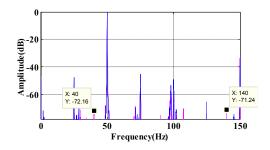
Fig.12. Second test of stator current spectrum of healthy (blue) and faulty (purple) motor at no load by FFT technique with outer raceway defect (s=0).
