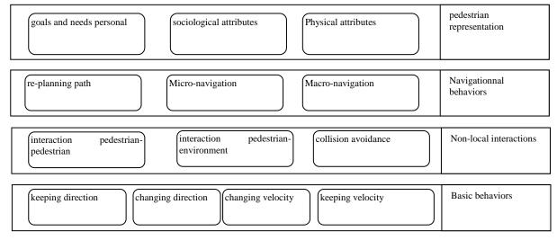
Figure 02: Hierarchical model for pedestrian behaviors
