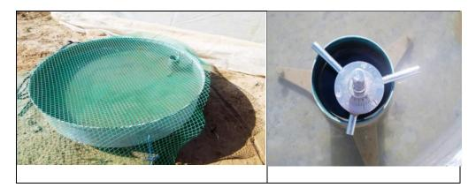
Figure 01: "Class A" evaporation pan(left) and level gauge (right)
