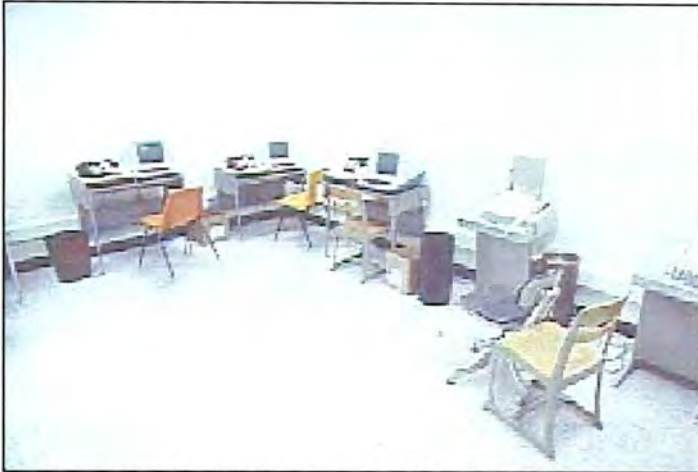
Public workstations in basement of Upson II. Note the telephones used for connecting the terminals to the mainframe.
