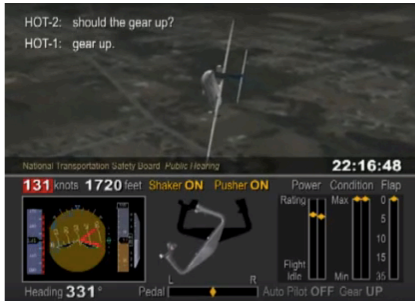
Figure 8. Flight 3407 – 10 Seconds form Impact - Final Roll to the Right and Pitch Down (NTSB, 2010)
