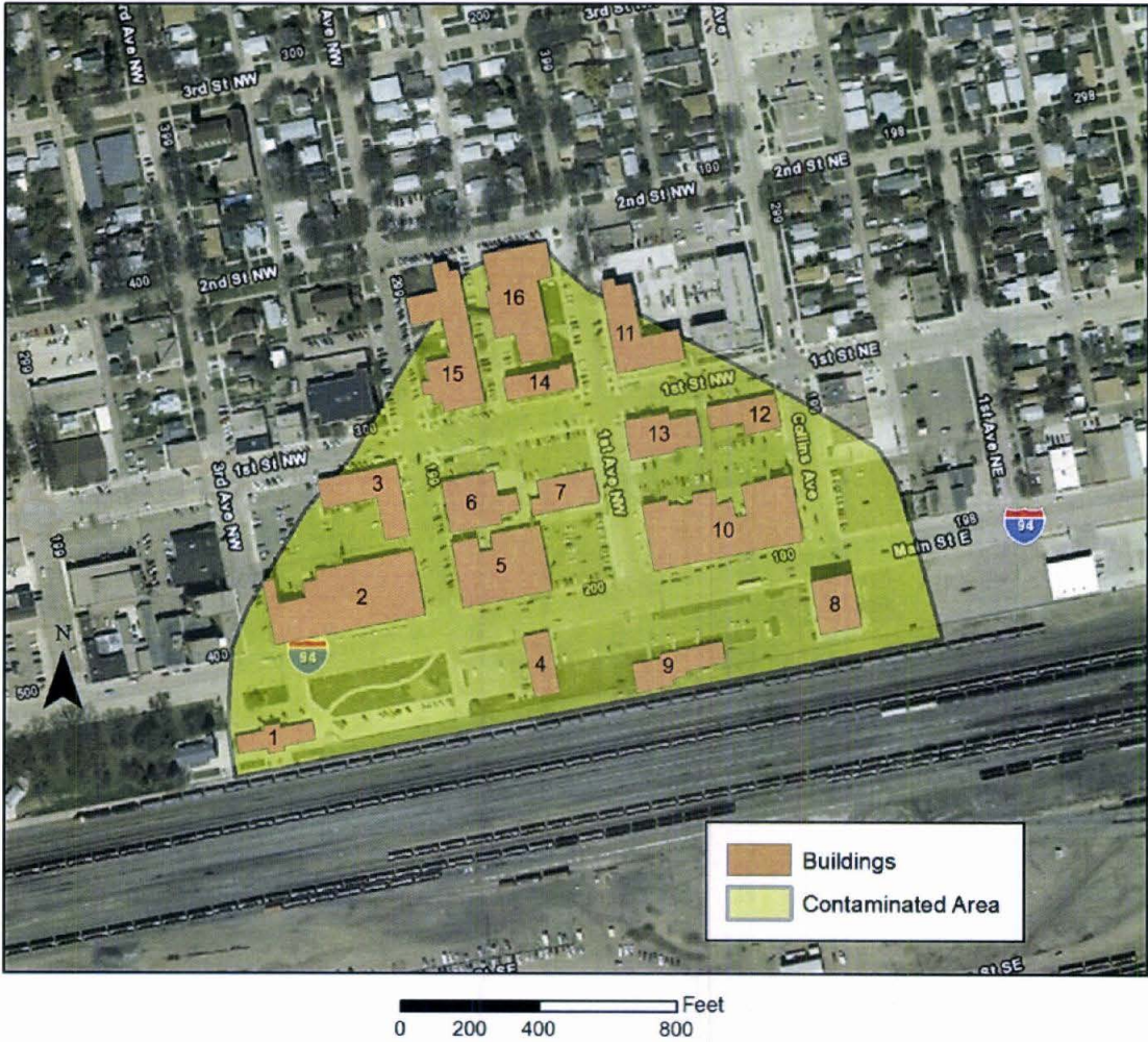
Figure 7 - Contamination zone with building locations
