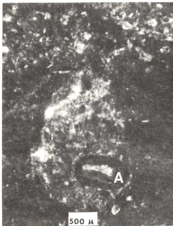
Fig. 26. Photomicrograph of a burrow in a mudstone filled by overlying packstone. Note ooliticly coated grain in burrow (A). Crossed nicols. Thin section No. 274-3339.
