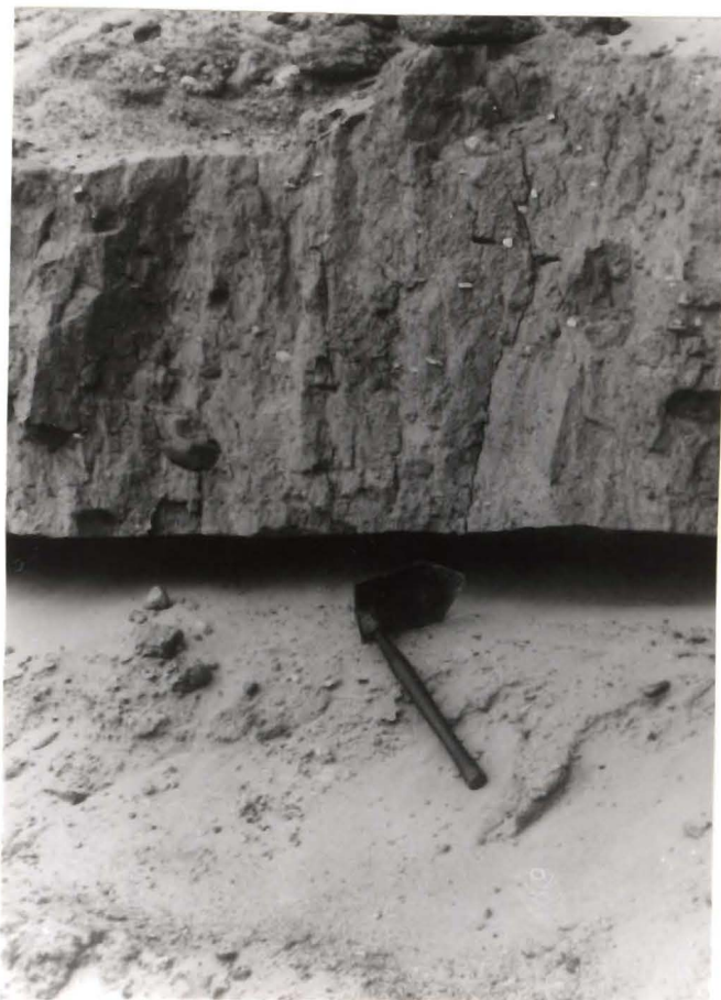
Figure 19. Contact between till and fluvial facies of the Mercer drift. Sand is loose and washes out easily leaving overhanging cliffs of Mercer till that tend to break off as large chunks and fall into the reservoir.
