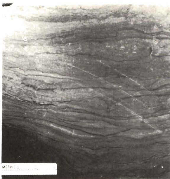
Fig. 25 --Core slab of wispy laminated, porous dolomitic mudstone. Note desiccation features along right-hand side.
