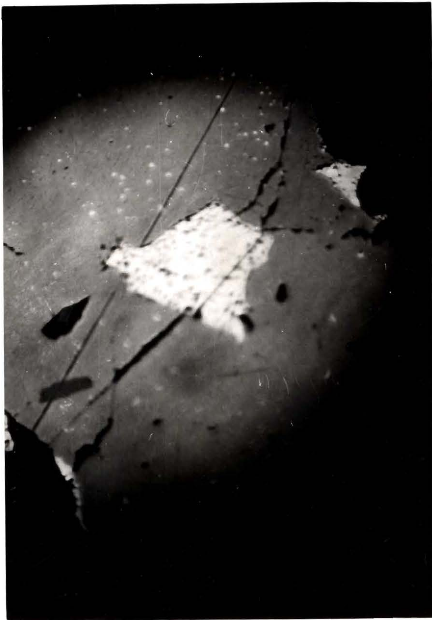
Figure 16. Exolution of chalcopyrite from sphalerite
