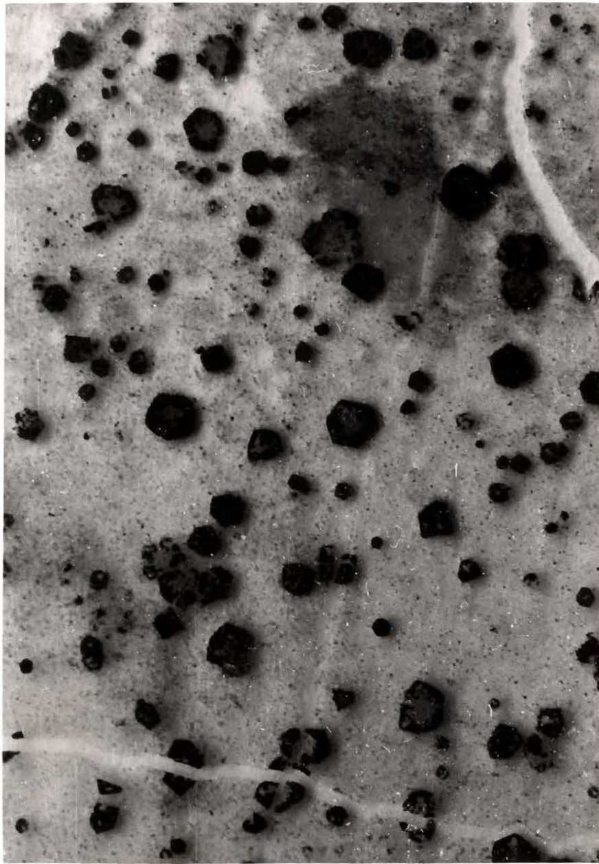
Figure 13. Spots of sulfides in country rock
