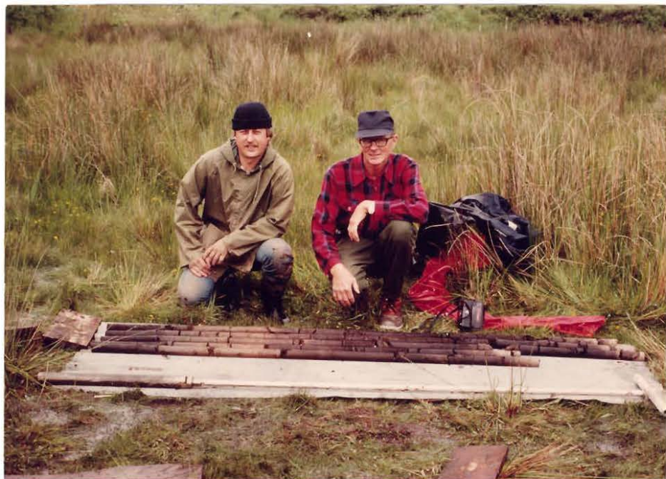
Figure 6. Photograph of the piston corer and some of the cores recovered from the Puerto Octay Site. The top of the cores is to the left. The dark layers are organic rich and the light contain volcanic ash. John Mercer is on the right and the writer on the left.
