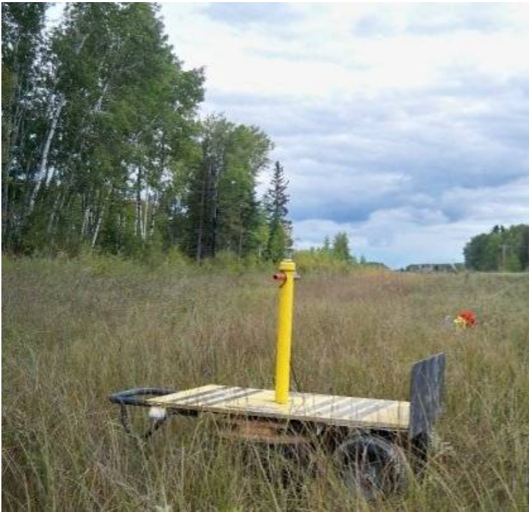
Fig. 23. The Ballistic Ordinance Seismic Source, (BOSS).
