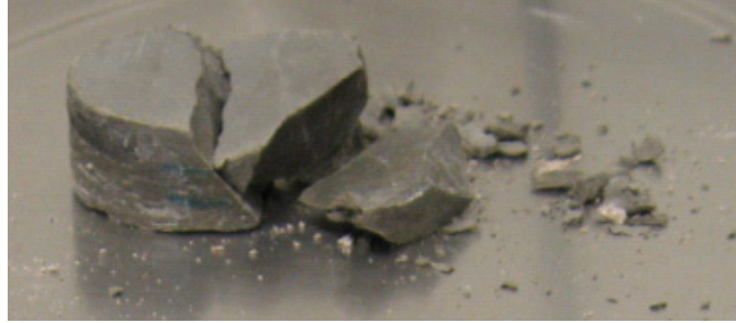
Figure 5.14. Rock deterioration after water flow followed by CO 2 flow
