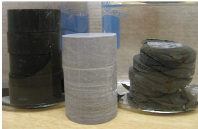
Figure 5.3. Changes of Pierre shale samples after contact with different fluids (crumbled in water (right), darkened in mineral oil but still intact (left), unchanged in air (middle))
