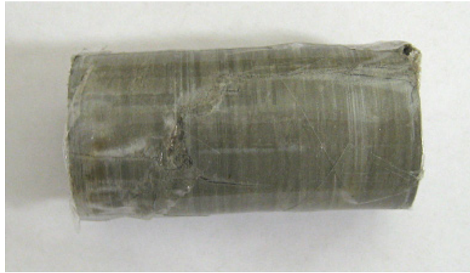
Figure 5.16. Rock sample after triaxial test (Sample 09PA05)
