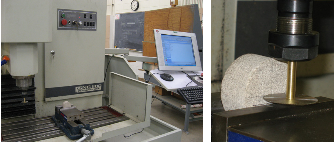
Figure 4.28. CCNBD specimen preparation
