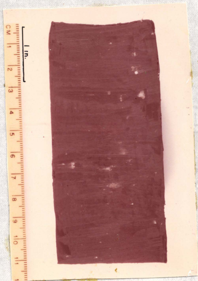
Figure 3. Unit 7 from Leonard Hall, Grand Forks. Gray clay with weathered carbonate pebbles. Does not appear stratified. Horizontal lines knife scrapings. Sample depth 63.5 feet.
