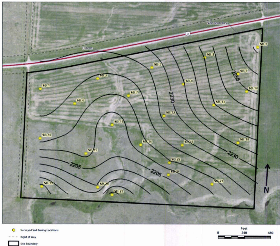
Figure 9. A topographic map of the WISCO Oil Field Landfill Site detailing the northeast to southwest sloping trend. (Barr Engineering, 2014)
