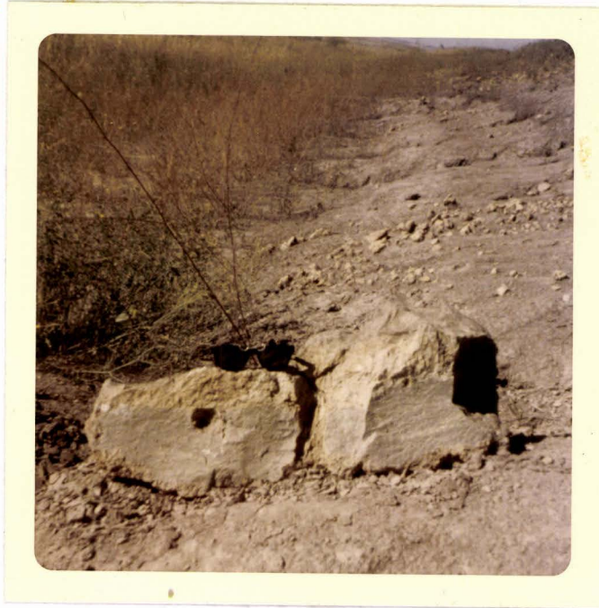
FIG. 7. -- SILICEOUS ROCK EXHIBITING LIGHT BROWN, WEATHERED RIND, ADAMS COUNTY, T130N R98W. NOTE ROOT CAVITY IN SAMPLE ON THE LEFT.
