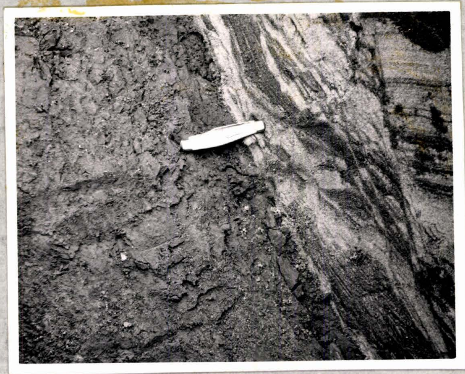
Fig. 15.- Sharp contact of organic-rich lake sediment and stratified quartz sands at Homme Reservoir site.
