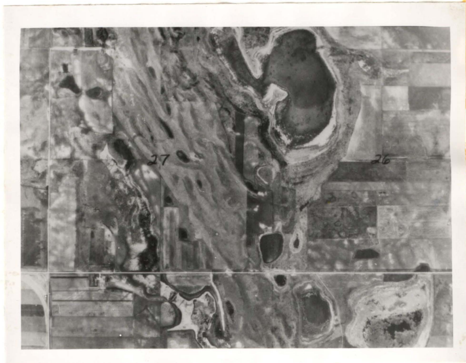
Figure 12. Southern portion of the Cooperstown end moraine showing linear ice thrust ridges and other features. Sections 22 and 27, T. 147 N., R. 60 W.
