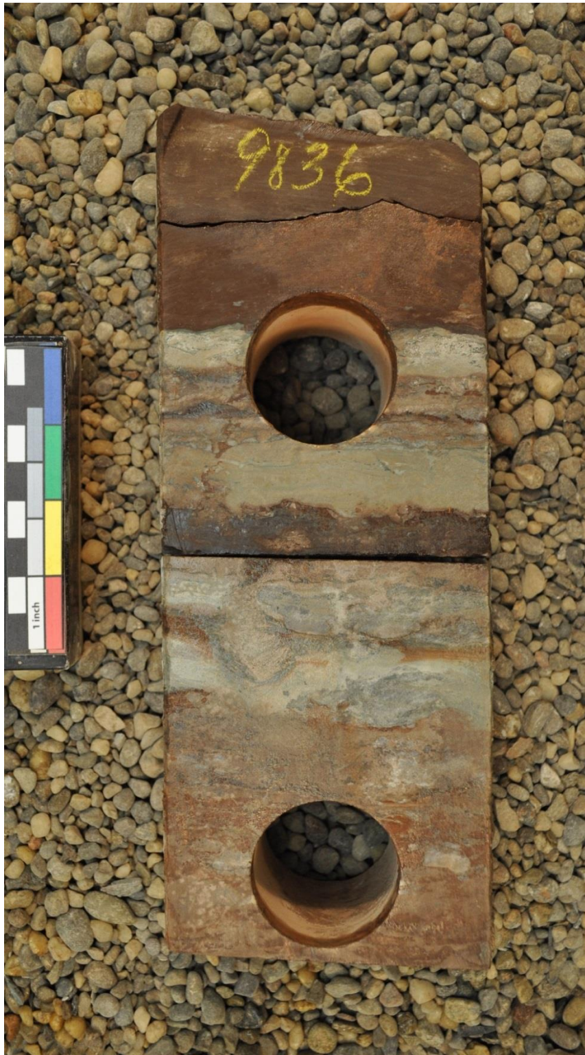
Figure 8. Three Forks Lithofacies G. (Core depth of 9836', NDIC Well #18101, API #33-061-01027-00-00, SESE 11-151-91)
