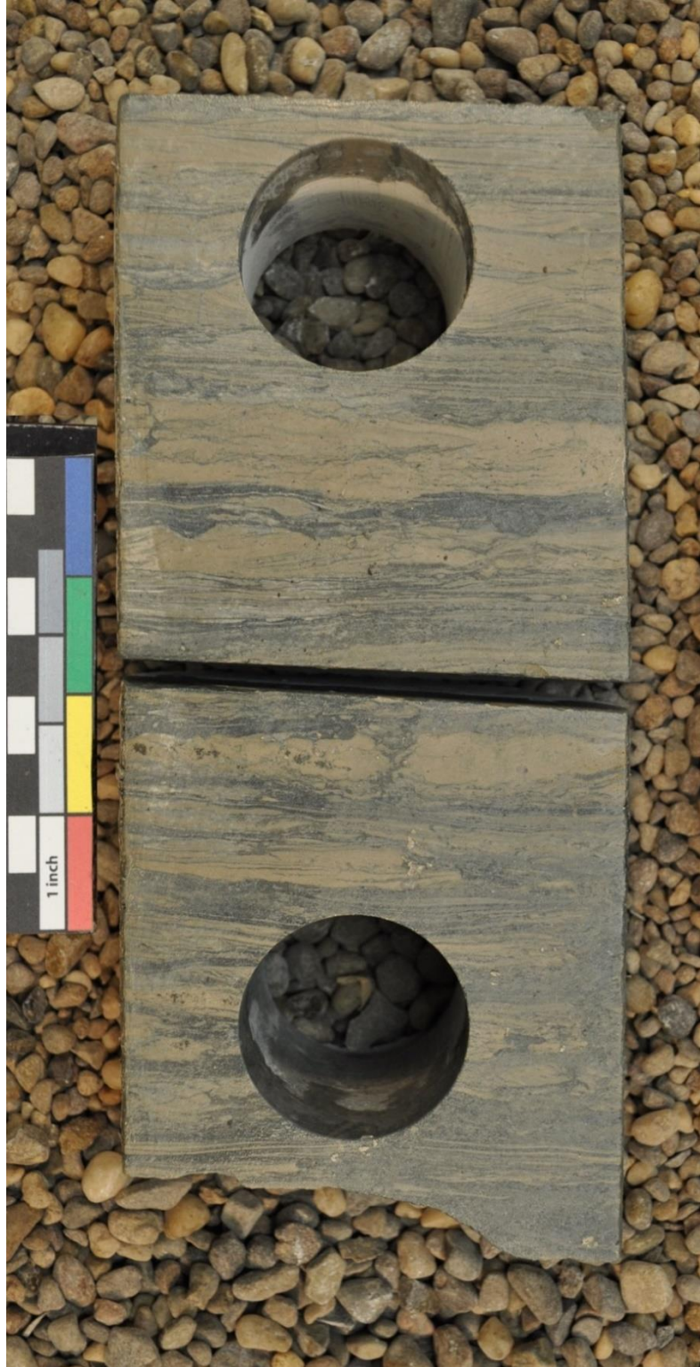
Figure 2. Three Forks Lithofacies A. (Core depth of 9703', NDIC Well #18101, API #33-061-01027-00-00, SESE 11-151-91)
