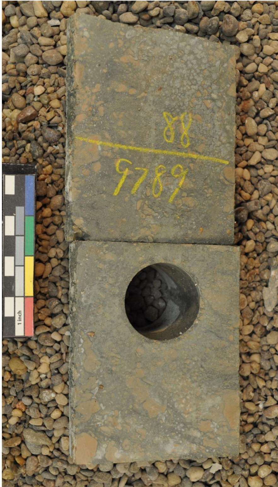
Figure 5. Three Forks Lithofacies D. (Core depth of 9789', NDIC Well #18101, API #33-061-01027-00-00, SESE 11-151-91)
