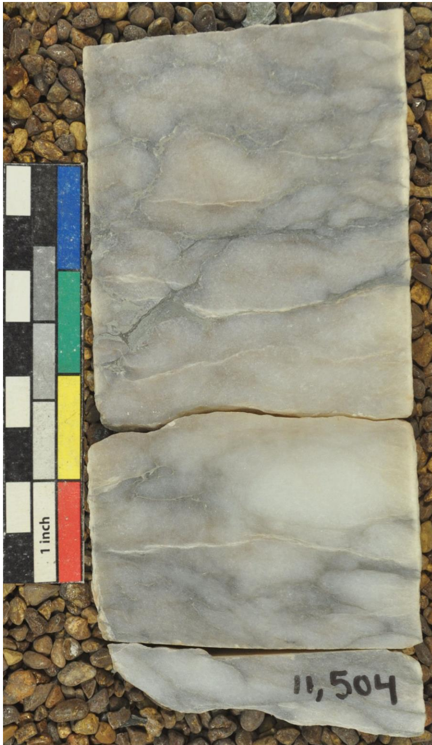
Figure 10. Three Forks Lithofacies I - Bed of "chicken wire" anhydrite in the lower Three Forks. (Core depth of 11504' corresponding to a log depth of 11510', NDIC Well #18101, API #33-061-01027-00-00, SESE 11-151-91)
