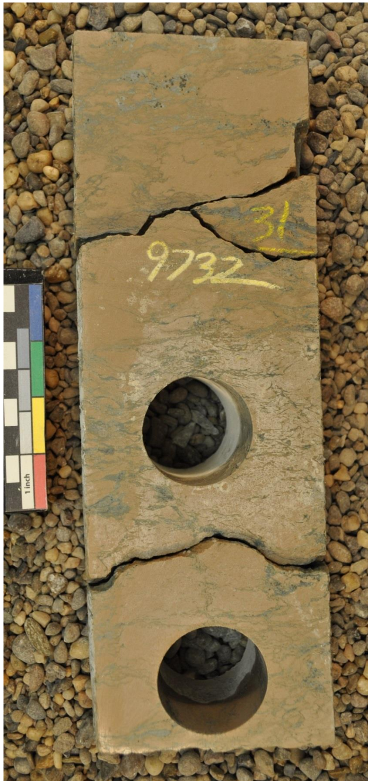
Figure 3. Three Forks Lithofacies B. (Core depth of 9732' NDIC Well #18101, API #33-061-01027-00-00, SESE 11-151-91)
