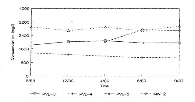
Figure 32. Monitoring nest 1 (undisturbed site) - sulfate concentration vs time. Pressure- vacuum lysimeters (PVL) 3, 4, and 5 are located at depths of 5, 10, and 15 feet (1.5, 3.0, and 4.5 m), respectively. Refer to Figure 3 for instrument locations.
