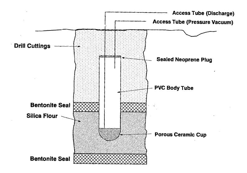
Figure 5. Monitoring nest schematic diagram.
