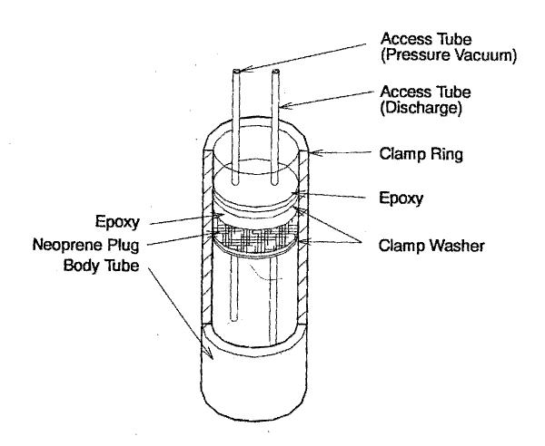
tamped into place at 1 foot (.3 m) intervals. A 4-foot (1.3 m) length of 4-inch (10 cm) PVC pipe was installed at the top of the borehole to house the access tubes. A vacuum of 28 inches of mercury (60 centibars) was pulled on the instrument to initiate sample collection. Vacuums were maintained periodically to insure adequate sample collection. Completion summaries for all the lysimeter installations are provided in Appendix B.
