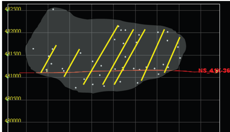
Figure 31. Map view of the induced fracture area (well NS 41X-36H) (Courtesy of BRC)
