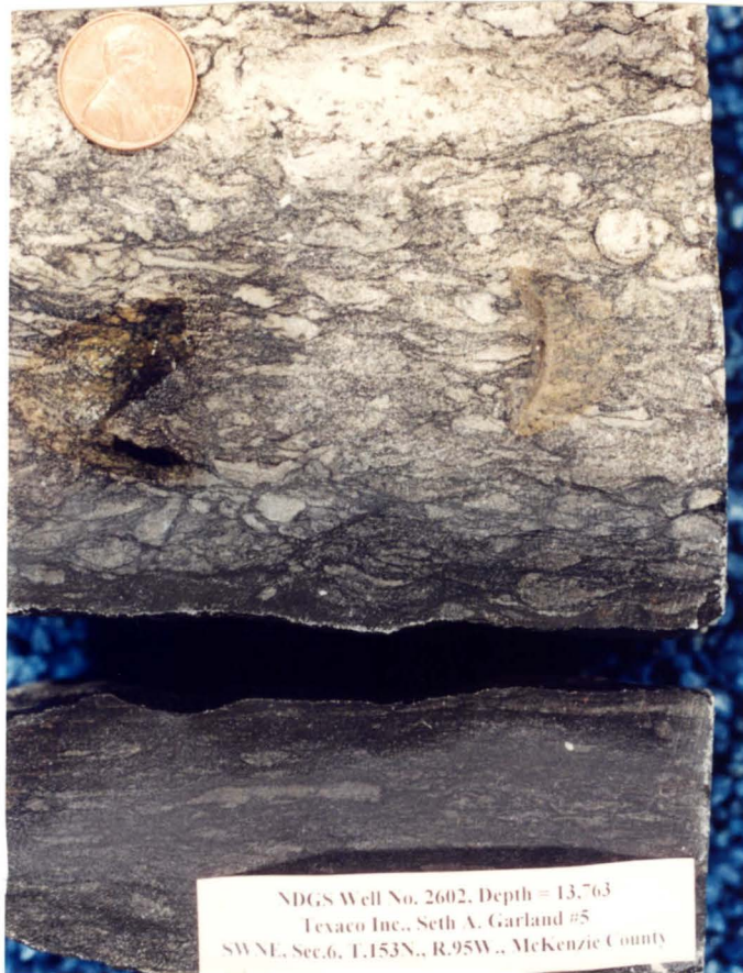
Figure 25. Gradation downward from bioturbated quartz arenite to clayshale within the bioturbated quartz arenite lithotype, Garland Member.
