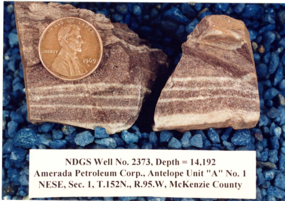
Figure 16. Thin beds of white quartz arenite interbedded within the red quartz arenite lithotype, Hawkeye Valley Member.
