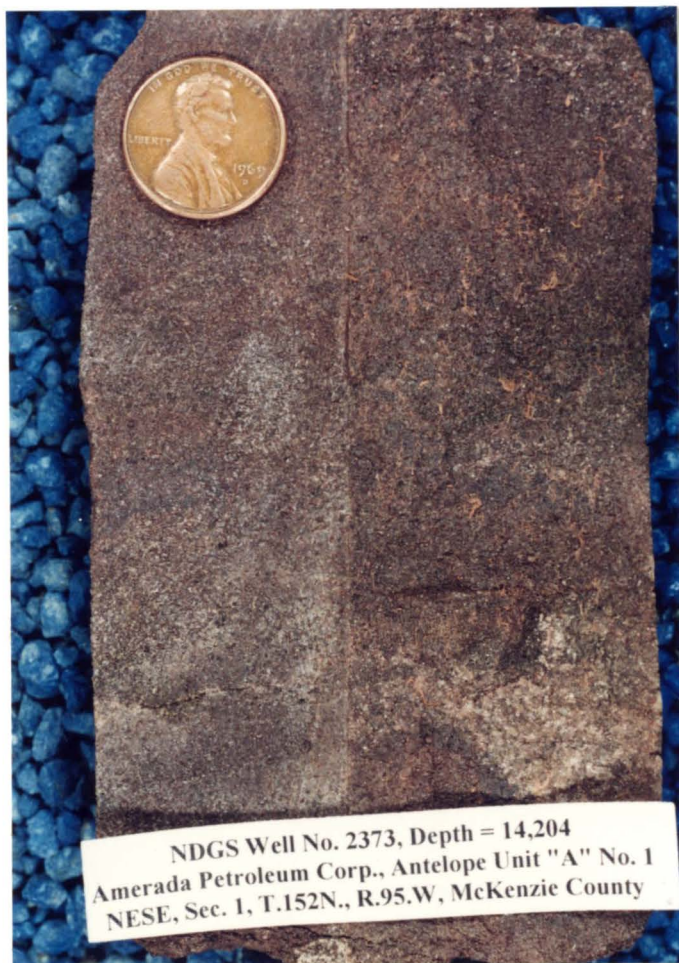
Figure 14. Core slab of dark reddish brown quartz arenite from the red quartz arenite lithotype, Hawkeye Valley Member.
