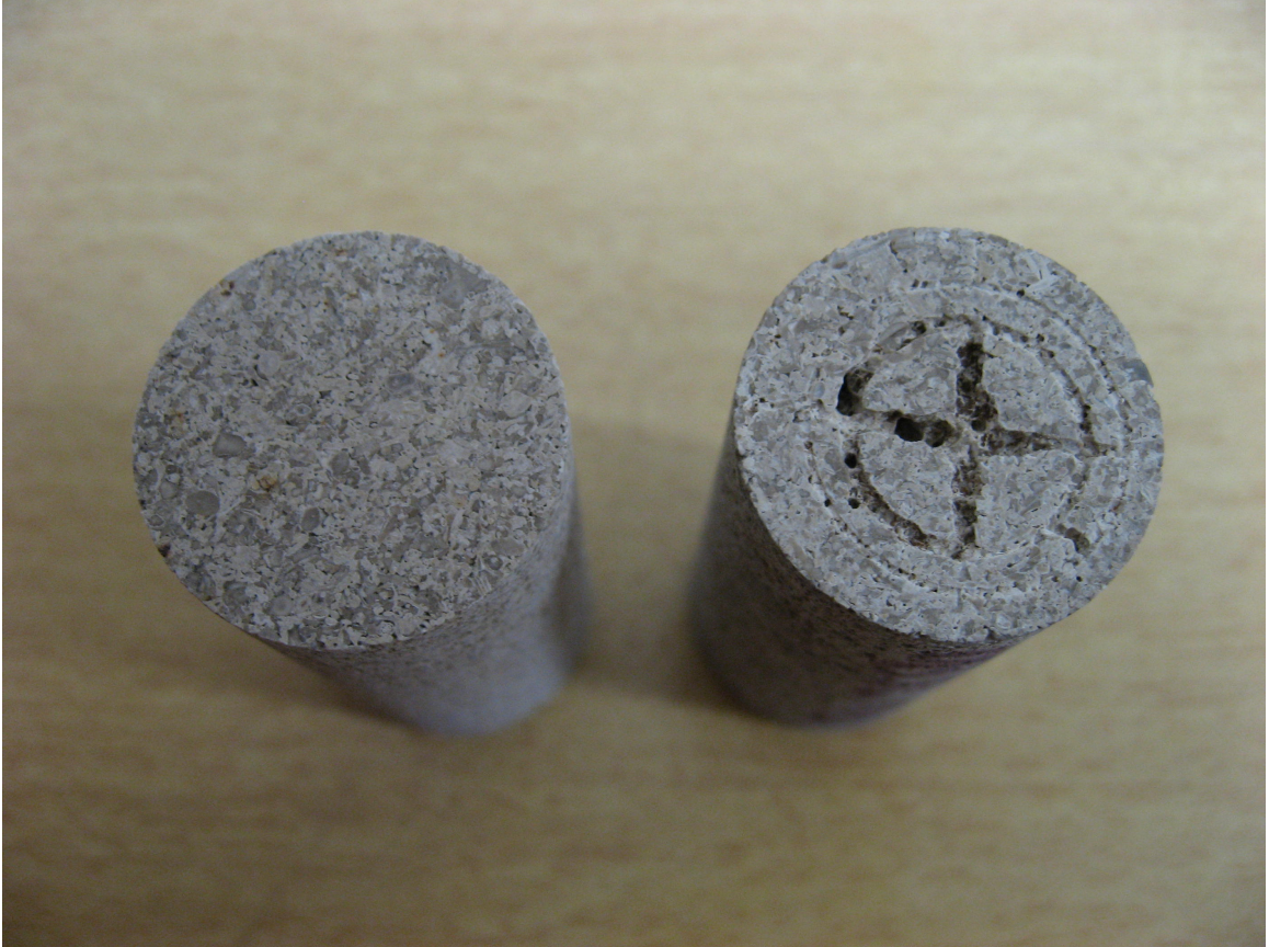
Figure 12. Limestone cores pre- and post-CO 2 flooding. Cores are from the 10,000 ppm experimental run, diameter is 2.54 cm.
