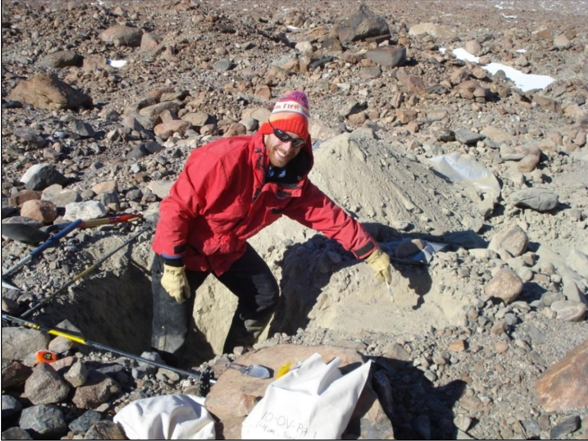
Figure 8. Typical field sampling procedure of bulk regolith. A pit is dug with shovel and intervals are sampled with hand trowel to depth.
