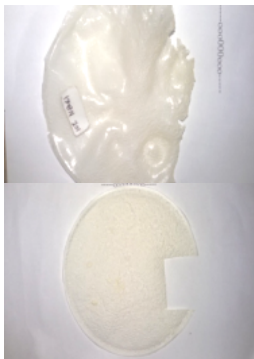
Figure 2. GPE test samples (A) without and (B) with plasticizer
