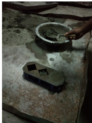
Figure 4: Preparation of Mortar
