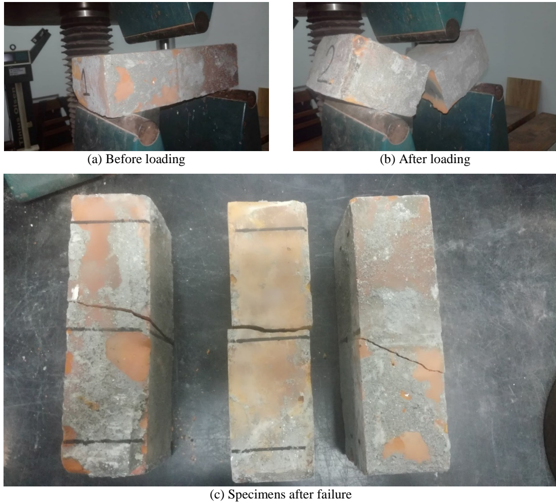
Figure 3: Modulus of Rupture Test of Bricks
