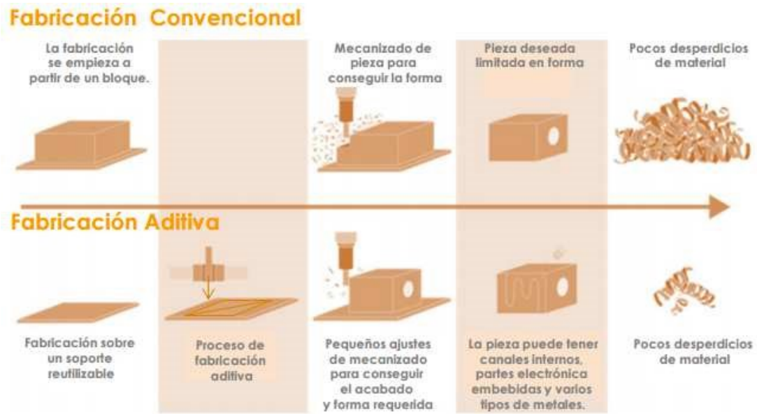
Figure 1: comparison between Conventional manufacturing and Additive manufacturing
