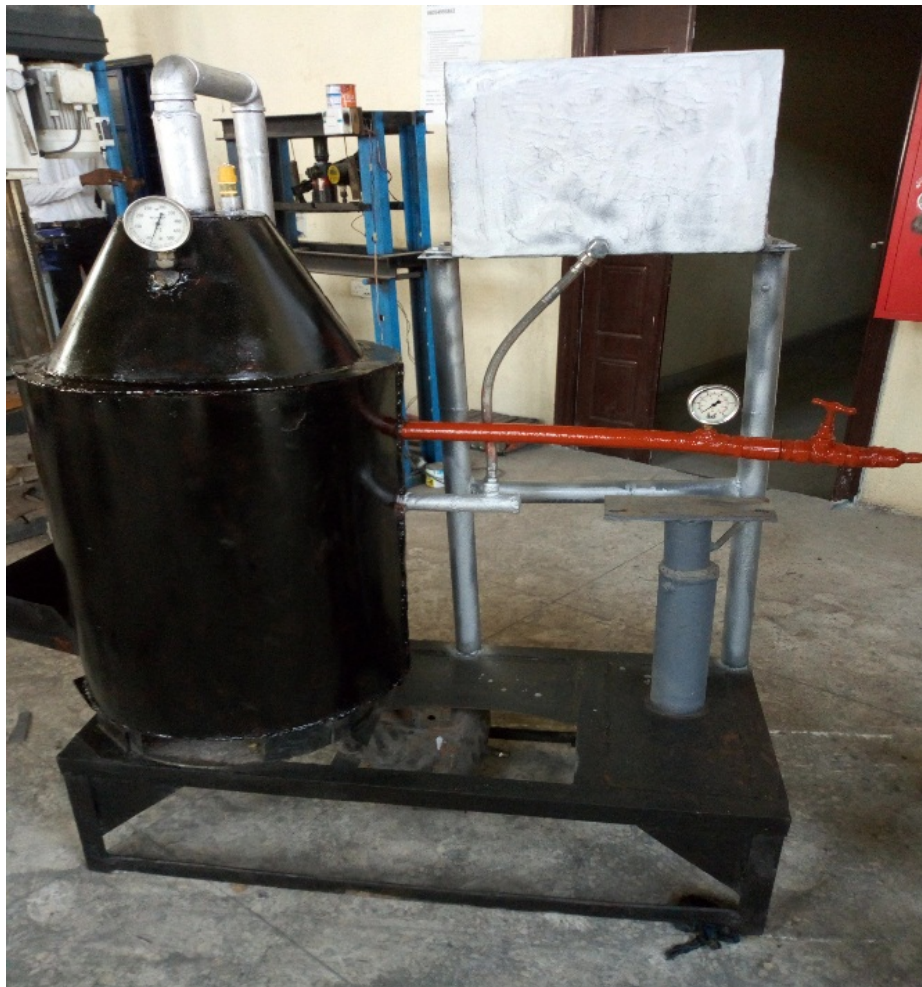
Figure 7: The fabricated boiler
