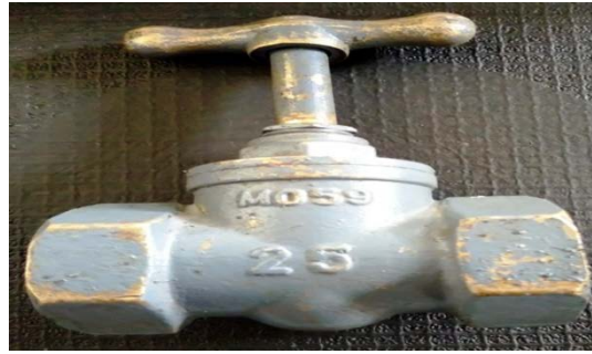
Figure 2: Selected Stopcock Gate Valve
