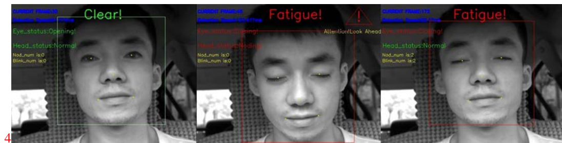
Figure 6: The screenshots of real-time fatigue driving detection on embedded platform
