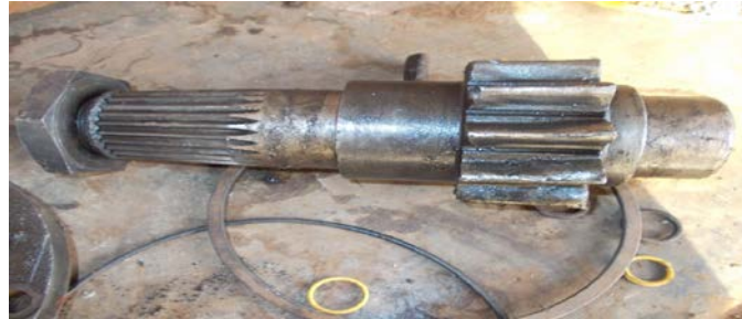
Figure 2: Repair Works on Pinion Bearing of Caterpillar Using E7018 Electrode
