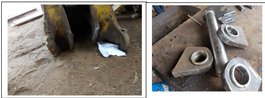
Figure 3: Back-hold Driller: Pieces Formed By Lathe. E6010electrode for Penetration and E7018 for Build Up
