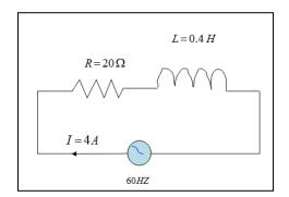
Figure 2: Impedance of the circuit
