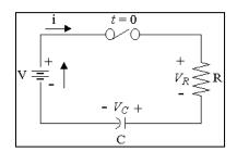
Figure 8: An RC series circuit
