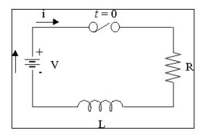
Figure 7: RL circuit diagram
