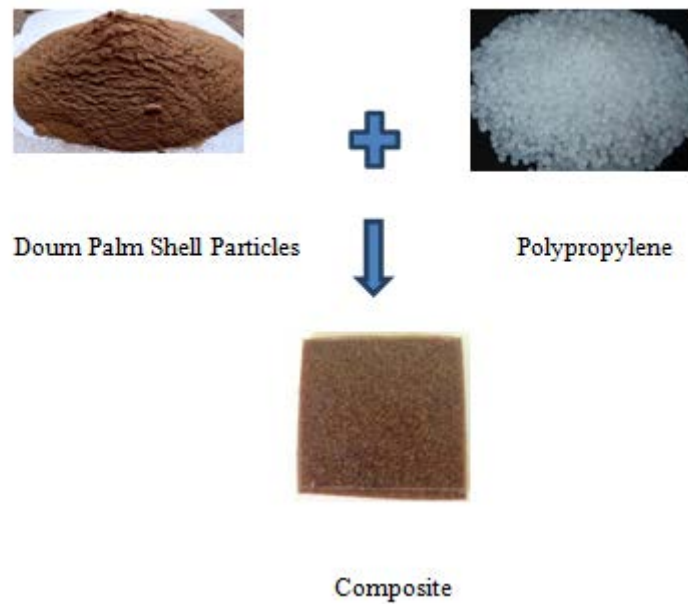
Figure 3: Doum palm shell particles and polypropylene Composite
