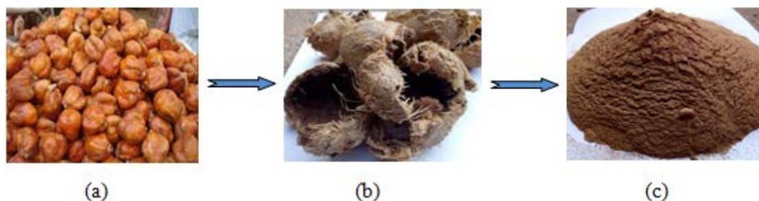
Figure 2: From doum palm fruit to doum palm particles. (a) Fruit (b) Shell and (c) Particles
