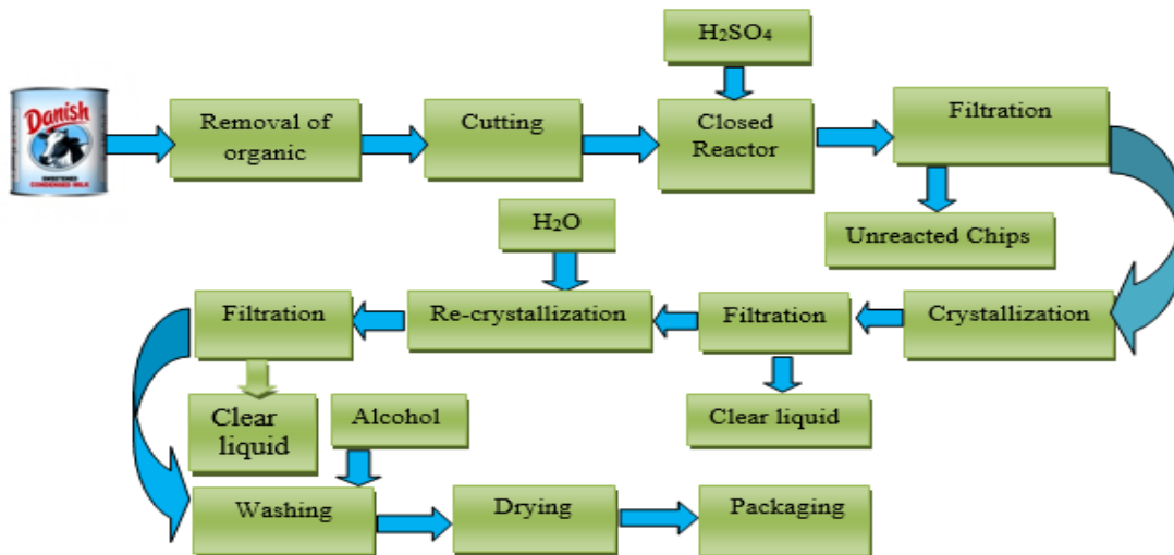
Figure 1: Flow-diagram for the production of ferrous sulphate
