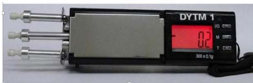
Figure 2: Digital yarn tension meter
