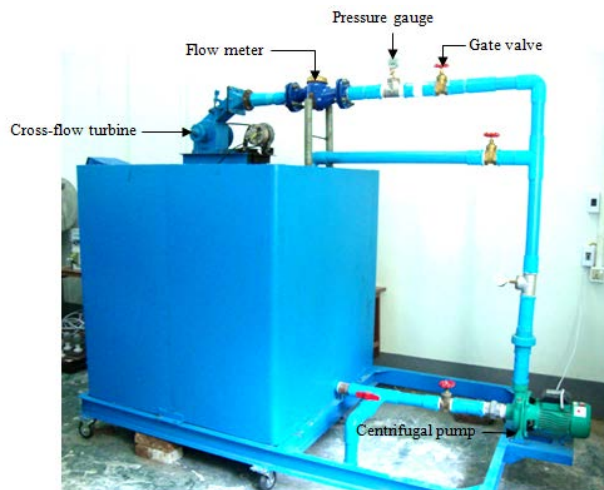
Figure 4: Experimental Set-up of Cross-flow Turbine
