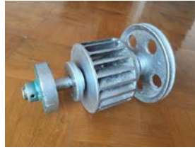
Figure 23: runner with pulley and flywheel
