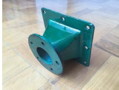
Figure 26: adapter used in cross-flow turbine
