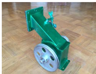
Figure 25: assembly of casing with runner and nozzle
