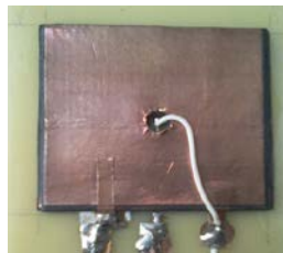
Figure 2: Photograph of integrated LC filter prototype
