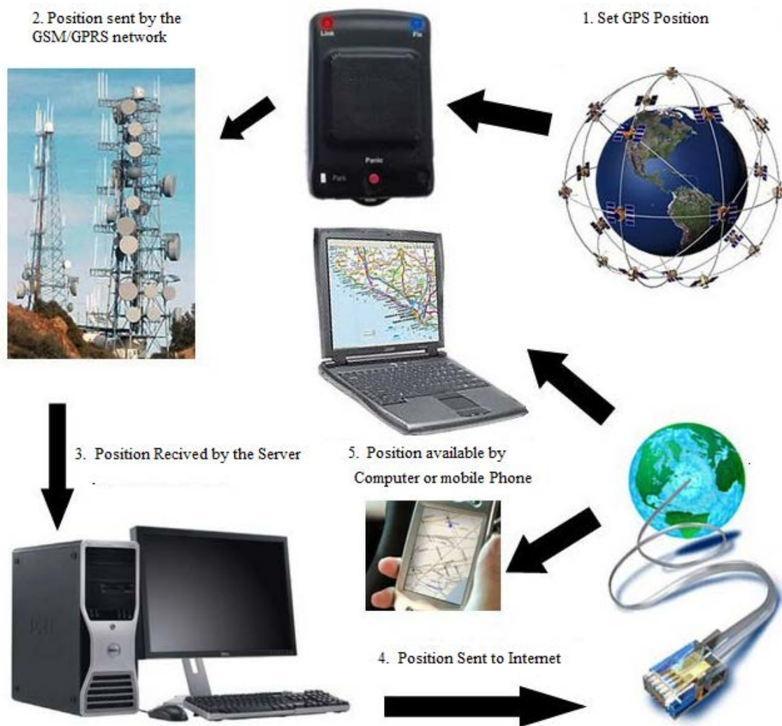
Figure 1: Global Connectivity with APRS-GSM-GPRS
