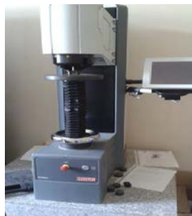
Figure 6: Macro hardness tester
