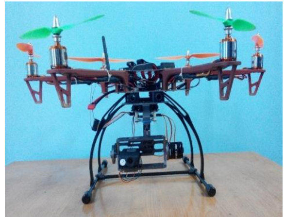
Fig.15 Stabilisation System Gimbal Camera on Hexacopter
