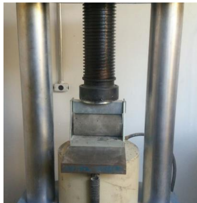
Figure 7: Diametral compression test for conventional and fiber reinforced concrete.
