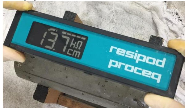
Figure 5 – Equipment used to test surface electrical resistivity.
