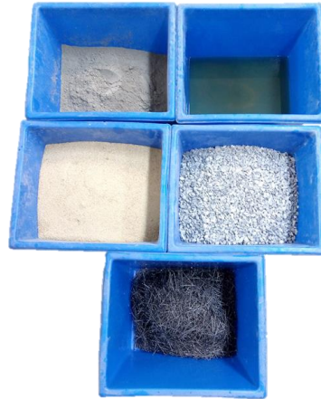
Figure 3: Materials used in preparation of concrete.
