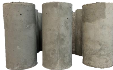
Figure 4: Concrete cylindrical specimens after demolding.
