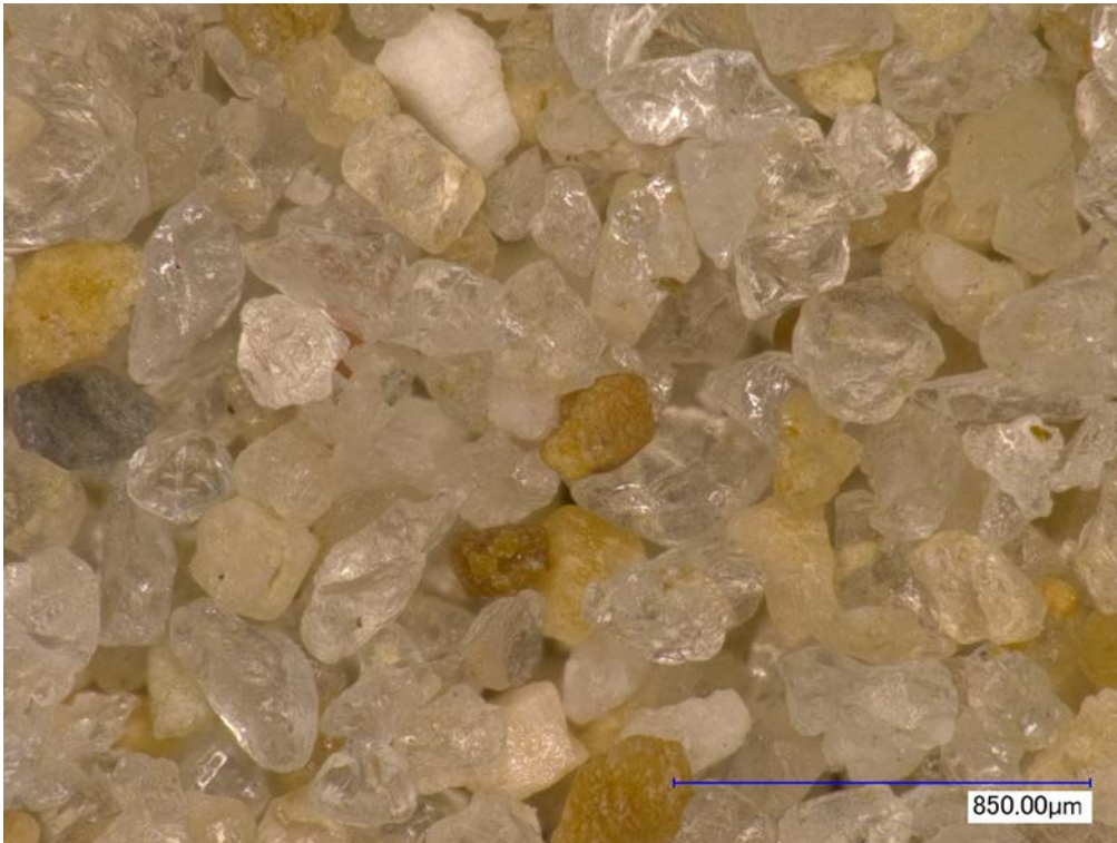
Figure 3.2-2 Microscope photographs of tested materials - Toyoura Sand
