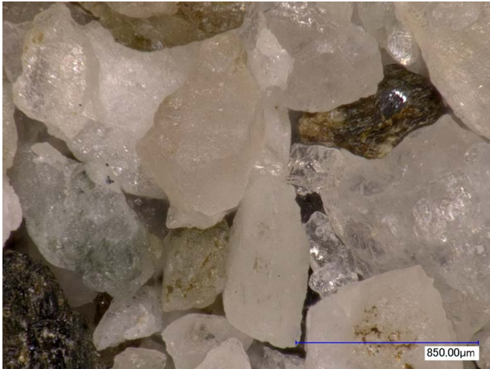
Figure 3.2-4 Microscope photographs of tested materials - Takasegawa sand
