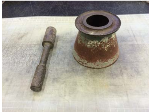
Figure 3.3-12 A photo of The assembly of the apparatus for water absorption of fine aggregates
