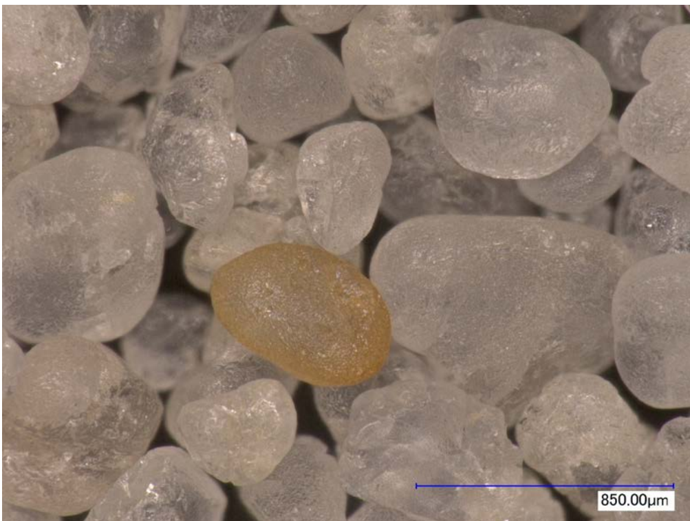
Figure 3.2-3 Microscope photographs of tested materials - JCA Sand
