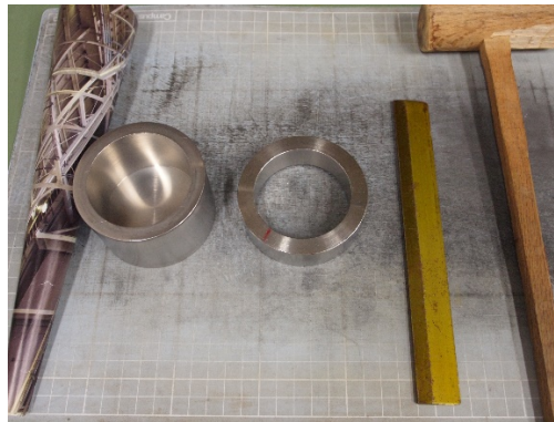
Figure 3.3-10 A photo of the assembly of the apparatus for the minimum and maximum densities of the sands
