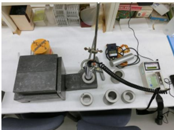
Fig. 8-3 The measurement of the attenuation rate of the probe shield in the radiation controlled area is shown. The probe of the survey meter was set up at the position where the radiation dose rate was 21.30 \mu\text{Sv/h} . The probe was inserted into the probe shield, and then the radiation dose rate was recorded. The height of the probe shield was increase from 3 cm to 12 cm. The attenuation rate of the each probe shield was calculated.
