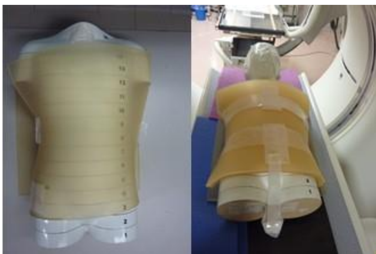
Fig. 4-4 The state of the child phantom wrapping with the layers of the material
