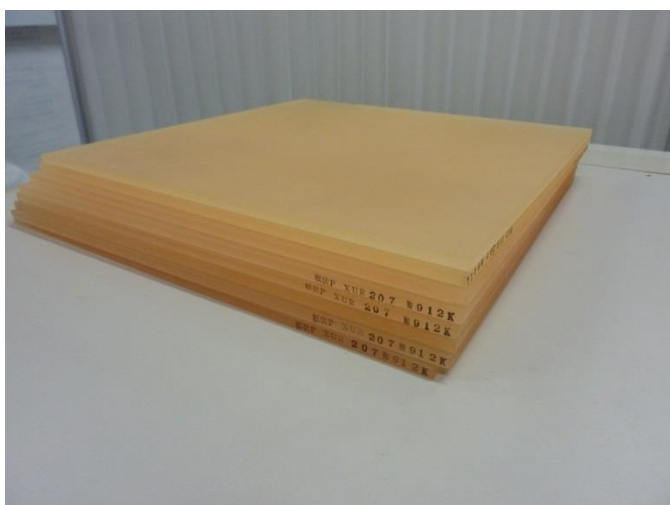
Fig. 4-3 The flat layers of soft-tissue-equivalent material
