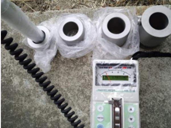
Fig. 8-4 The measurement of the attenuation rate of the probe shield at Kooriyama City is shown.
