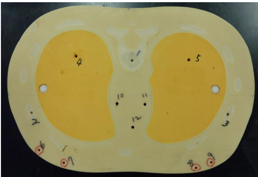
Fig. 3-3 One of the thick axial slices of the phantom.
