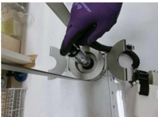
Fig. 8-5 The combination of the probe shield and the main shield is shown. The probe shield was attached to the main shield, and the probe of the survey meter was inserted into the probe shield.
