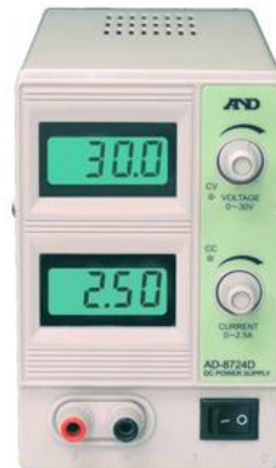
Photo. 7-6 The DC power supply
